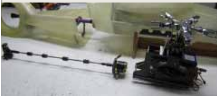
Main Rotor and Fantail Drive Relative to Aircraft
