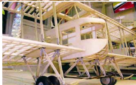
The wing and tail airfoil structure, nose cockpit, and landing gear technique is shown in these three photos
